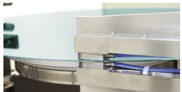
Wafer thickness measurement with two capacitive sensors
