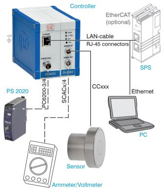
Fig. 13 Measuring system assembly
