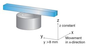
Fig. 31 Example of measuring range deviation in the case of a sensor distance of 100 % of the measuring range
