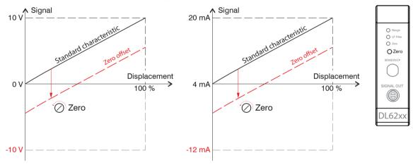
Fig. 14 Zero point shifting with zero-poti
