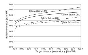
Fig. 33 Measuring value deviation in the case of measurement on ball-shaped targets
