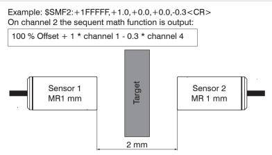
Fig. 22 Example for thickness measurement of a target with two capacitive sensors
