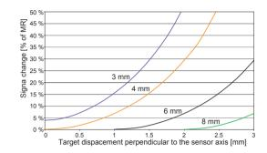
Fig. 30 Example of measuring range deviation in the case of a sensor distance of 50 % of the measuring range
