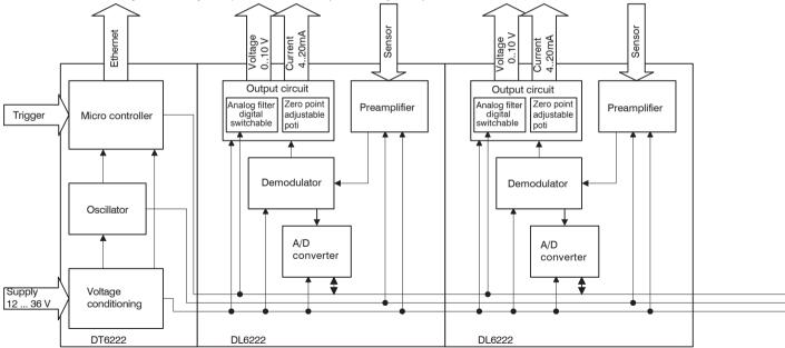
Fig. 2 Block diagram capaNCDT 6222
