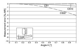
Fig. 28 Example of measuring range deviation in the case of a sensor distance of 100 % of the measuring range
