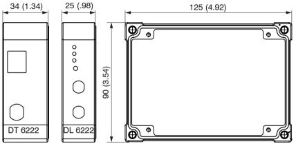
Fig. 6 Dimensional drawing controller
