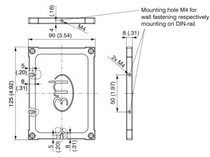
Fig. 7 Dimensional drawing housing cover
