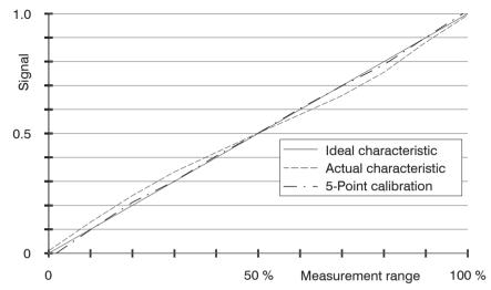
Fig. 21 Output characteristic for the measurement
