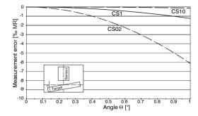
Fig. 27 Example of measuring range deviation in the case of a sensor distance of 50 % of the measuring range
