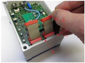
Fig. 10 Use of the plugging off assistance for the wiring of the demodulator elements
