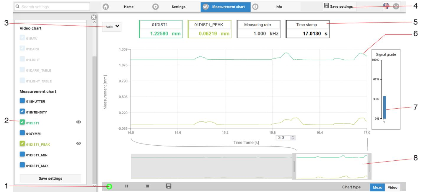
Fig. 37 Measurement (distance measurement) web page
