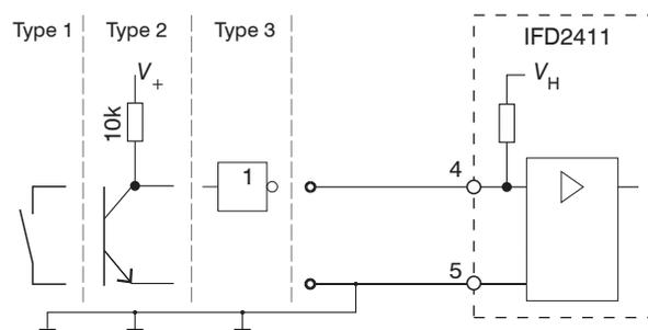
24V logic (HTL): Low  $\leq 3$  V; High  $\geq 8$  V (max 30 V),
