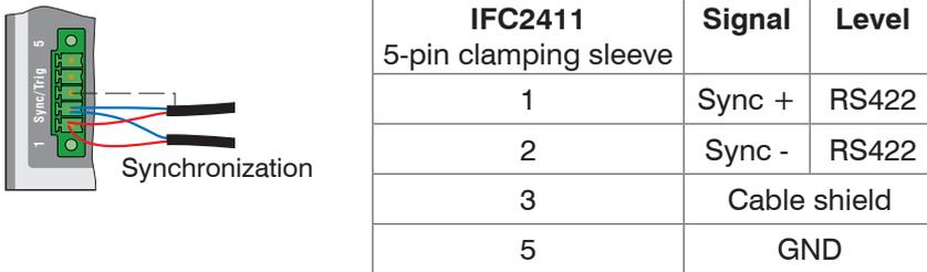
Fig. 26 Connections and signal level internal synchronization
