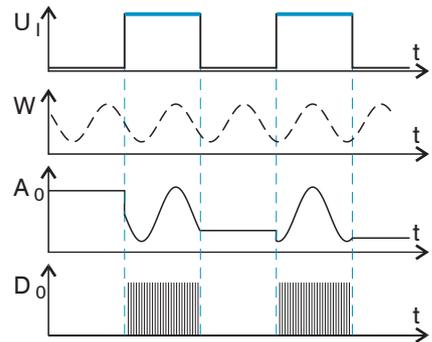
Edge triggering. Starts measured value input/output as soon as the selected edge is active to the trigger input. The pulse must be at least  $5 \mu\text{s}$ .
