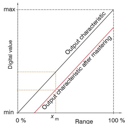
When setting a master, the output characteristic is moved in parallel. Moving the characteristic reduces the relevant measuring range of a sensor (the further master value and master position are located, the greater the reduction).
