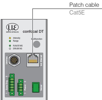
➡ Connect the IFC2411 and network with a shielded Ethernet cable (Cat5E, 2 m patch cable from the scope of delivery, total cable length shorter than 100 m).
