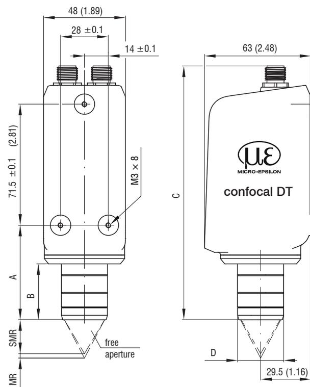
Fig. 5 Dimensional drawing IFD2410 | IFD2415, dimensions in mm
