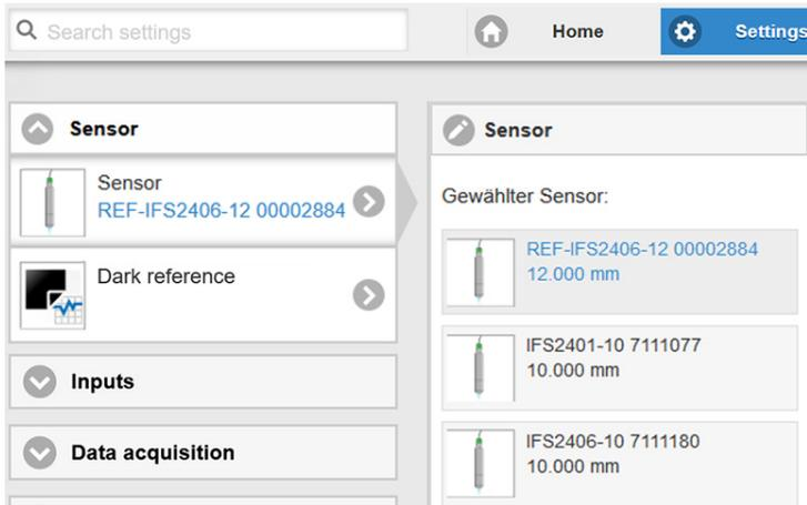
The calibration data of up to 20 different sensors can be saved in the controller. Calibration is only possible at Micro-Epsilon.
