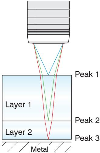
The refractive index needs to be corrected in the controller for an exact distance or thickness measurement.
