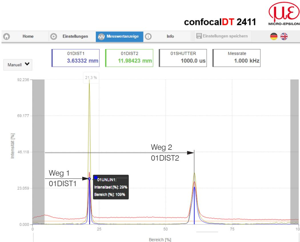
Fig. 72 Video signal web page, One-sided thickness measurement
