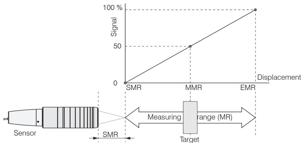
Fig. 1 Measuring range and output measuring system
