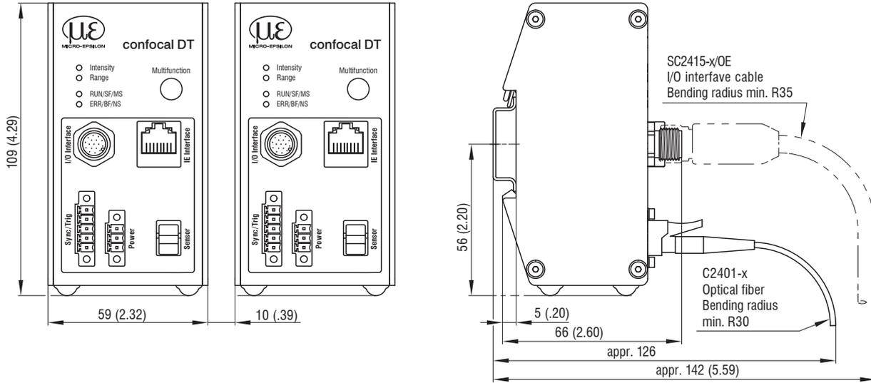
Fig. 19 IFC2411 dimensional drawing, dimensions in mm
