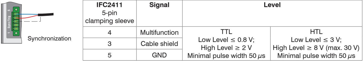
Fig. 28 Connections and signal level external synchronization
