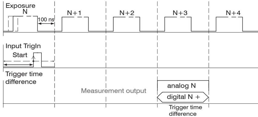
Fig. 44 Definition of the trigger time difference
