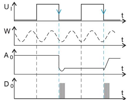
Software triggering. Starts data recording as soon as a software command (instead of the trigger input) or the Initiate trigger button is activated.
