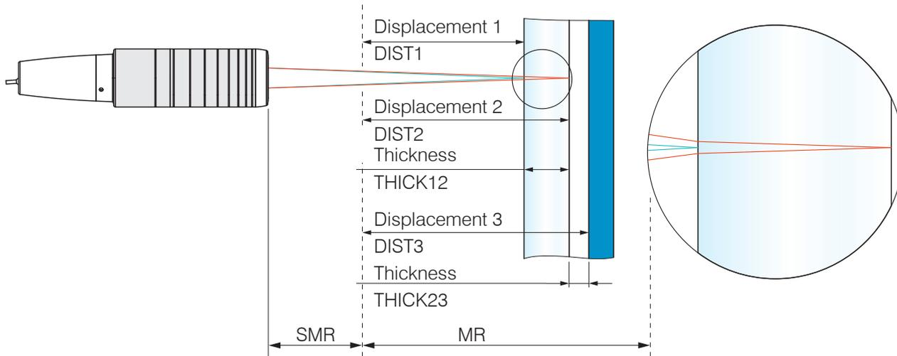
Fig. 71 One-sided thickness measurement on a transparent target
