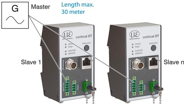
Fig. 29 Synchronization of multiple controllers, star-shaped
