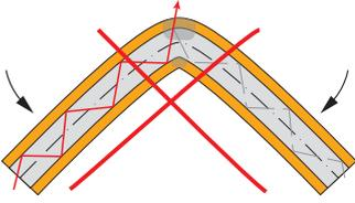
Do not pull the sensor cable over sharp edges.
