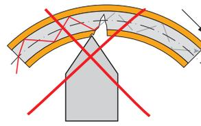
Do not crush the sensor cable, do not use cable ties to secure it.
