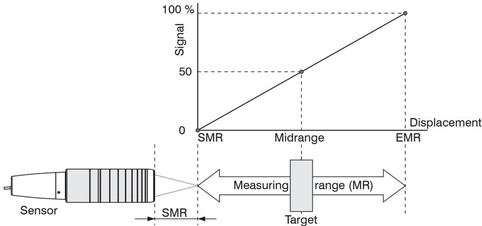
Fig. 41 Defining measuring range and output signal
