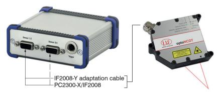
The 4-channel RS422/USB converter with trigger input is designed for one to four optical sensors with RS422 interface. The data is output through the USB interface. The sensors are supplied through the converter.
