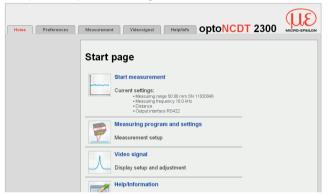
Programming the sensor. In the top navigation bar other auxiliary functions (settings, video signal, etc.) are available. All settings in the website will be immediately executed in the sensor after pressing the button Apply.
