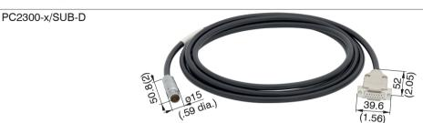
Power supply and output cable, x = length in m, drag chain suitable (x= 3, 6 or 9 m), for the supply with 24 VDC, signals: Ethernet, Ethercat, RS422, synchronization, laser on/off and limit switches
