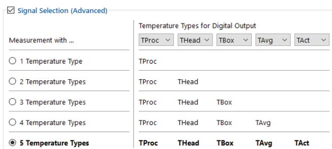
Fig. 7.11: Signal Selection (Advanced) with various options
