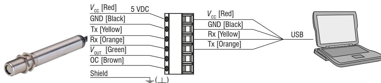
Fig. 6.4: Pin assignment digital output
