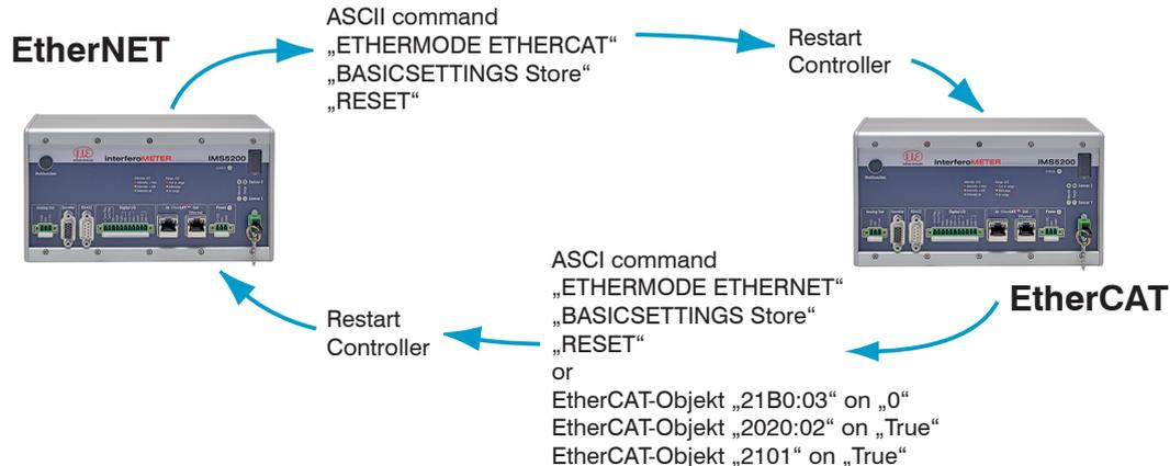
The RS422 interface for sending an ASCII command is available both in Ethernet mode and in EtherCAT mode.
