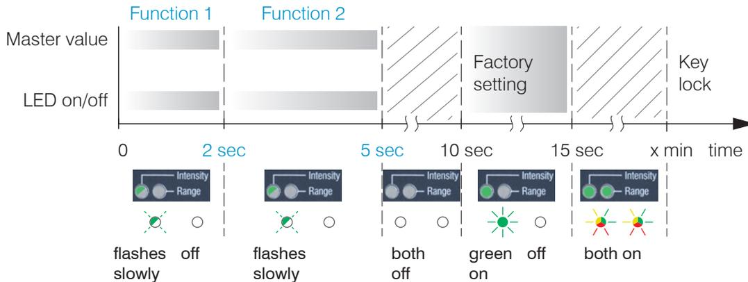
The Intensity and Range LEDs indicate the currently selected function.
