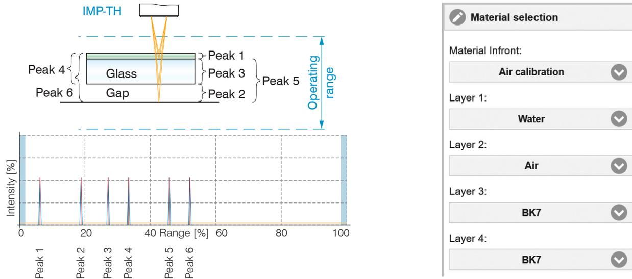
The IMS5200MP controller can also measure the thickness of combined layers of the same material.
