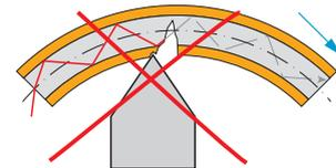
Please do not grind the optical fiber over sharp corners.
