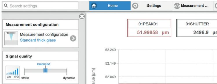
The signal quality is set to `Balanced` at the factory.
