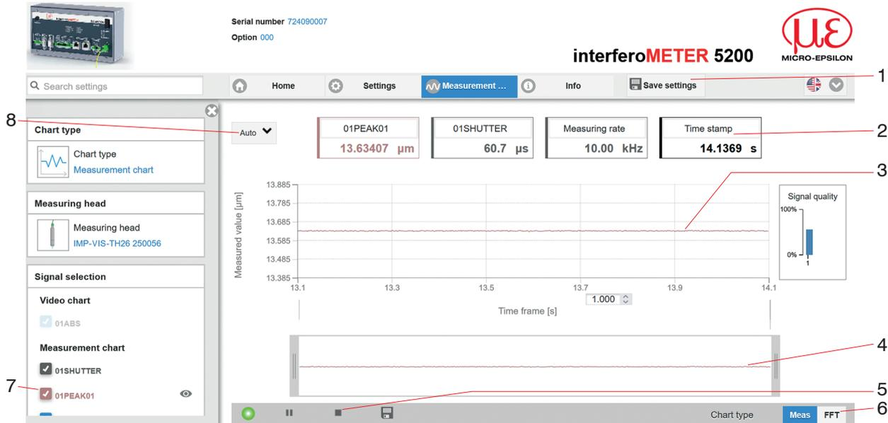
Measurement *web page (thickness measurement)*
