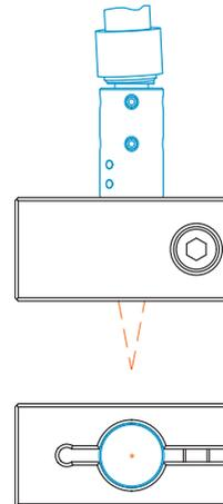
This type of sensor installation ensures the highest level of reliability because the sensor's cylindrical cover is clamped over a relatively large area.
