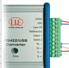
Symmetrical differential signals according to EIA-422, not electrically separated from the voltage supply. Use a shielded cable with twisted wires, e. g. PC3800-x. The RS422 interface can be used for configuration as well as for permanent data transmission, even over longer distances.
